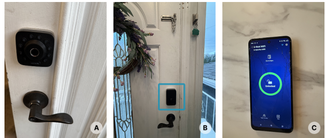
Figure 9: An example of the smart lock, two views from inside (A) and outside (B) of the door, that can be controlled by an app (C).
